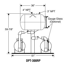
For a fully detailed certified drawing, refer to: SPT-400RP/DPT-400RP CDF #1005 SPT-3500RP/DPT-3500RP CDF #1046
